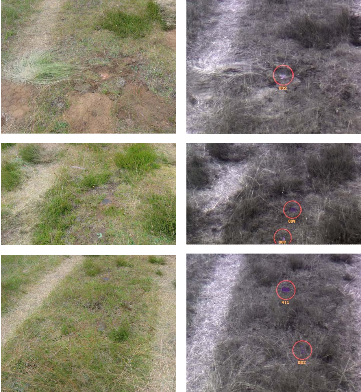
Figure 7 Examples of automatic detection results from buried mines. The images on the left show normal VIS pictures of the flush buried mines. The images on the right show the raw polarisation images with the visualisation of the detection results.
