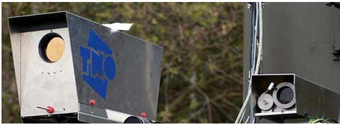
Figure 2 Different polarization measurement systems. From left to right a TIR system with a rotating polarizer, a VIS system with a rotating polarizer, and the layout of a VIS 3CCD system.
