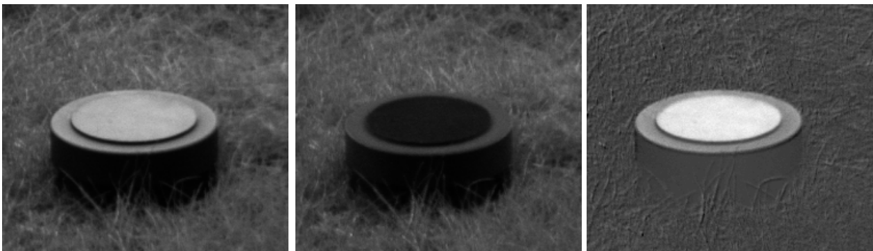
Figure 1 Example of the polarization effect on a dummy PMN mine in the visible light. The leftmost image is taken with a horizontal polarizer in front of the camera. The centre image is taken with a vertical polarizer and the third image is the difference between the two images. This last image clearly shows the polarization contrast between the mine and the background.
